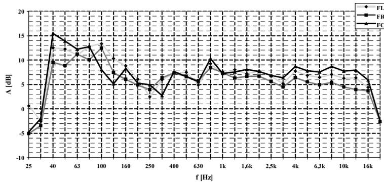
Fig.6. Measured operational room response curves (front channels)
