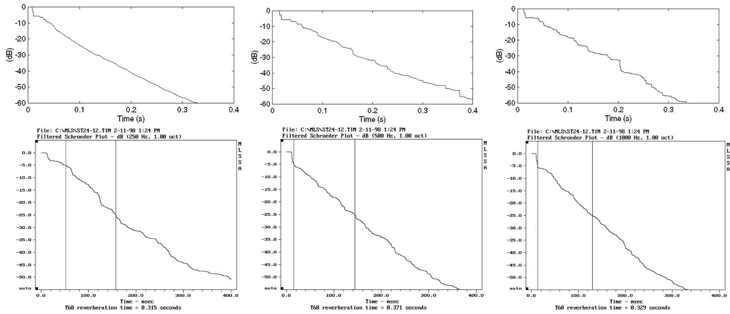
Fig.11. Measured and predicted Schroeder-plots (250Hz, 500Hz, 1kHz)
