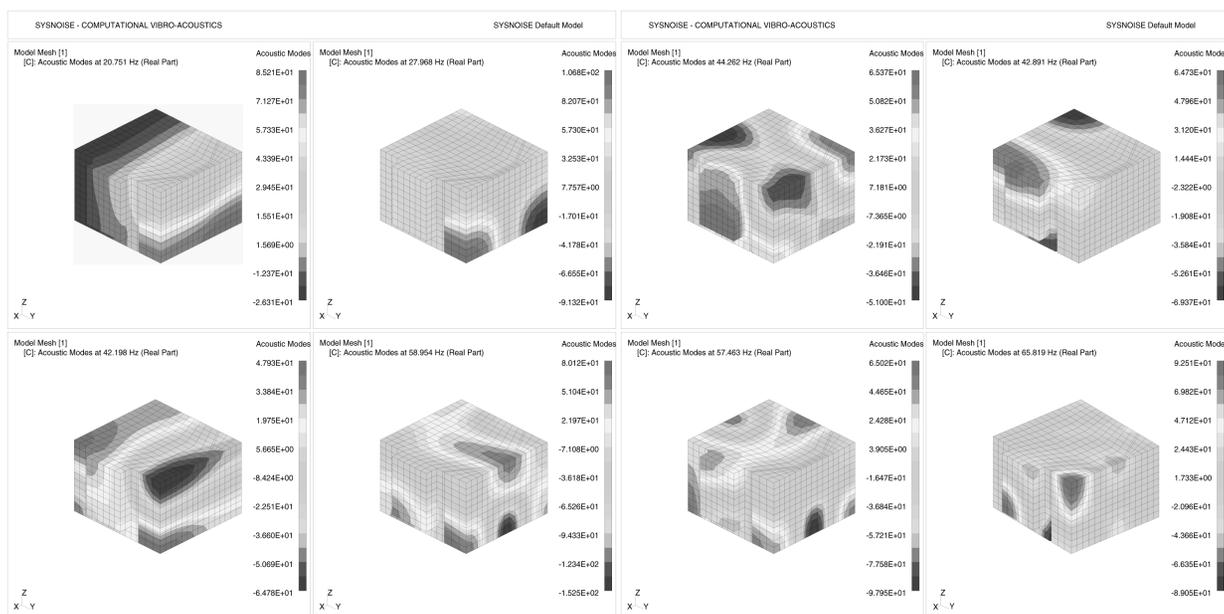
**Fig.2.** Examples of calculated room modes with FEM modeling (SYSNOISE).
