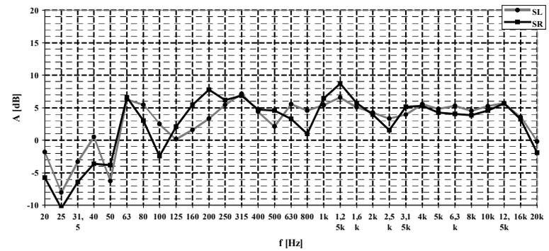
Fig.7. Measured operational room response curves (surround channels)
