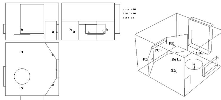
**Fig.1.** The floor plan and the 3-dimensional view of the listening room with the place of sound sources and the reference listening point. (FL - Front Left, FC - Front Center, FR - Front Right: Genelec 1038A; SL - Surround Left, SR - Surround Right: Genelec 1032A).
