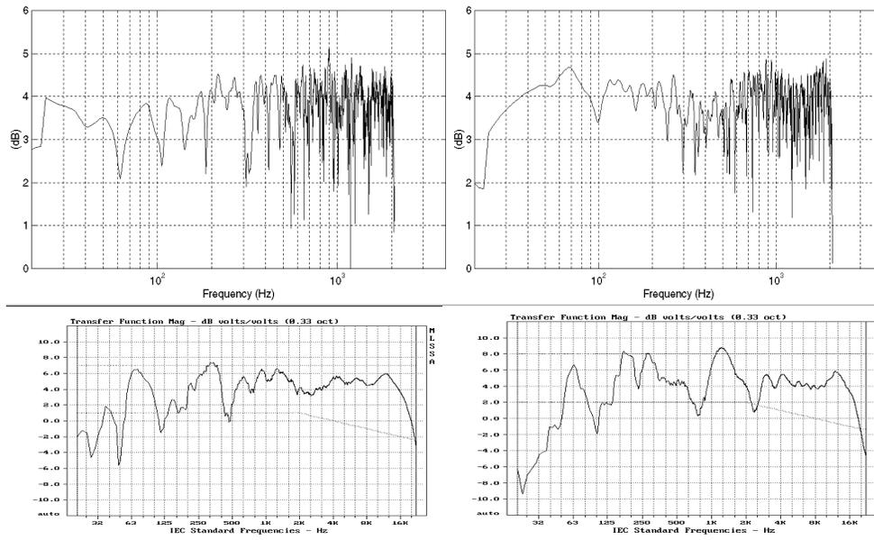
Fig.10. cont'd Measured and predicted transfer functions (SL, SR)
