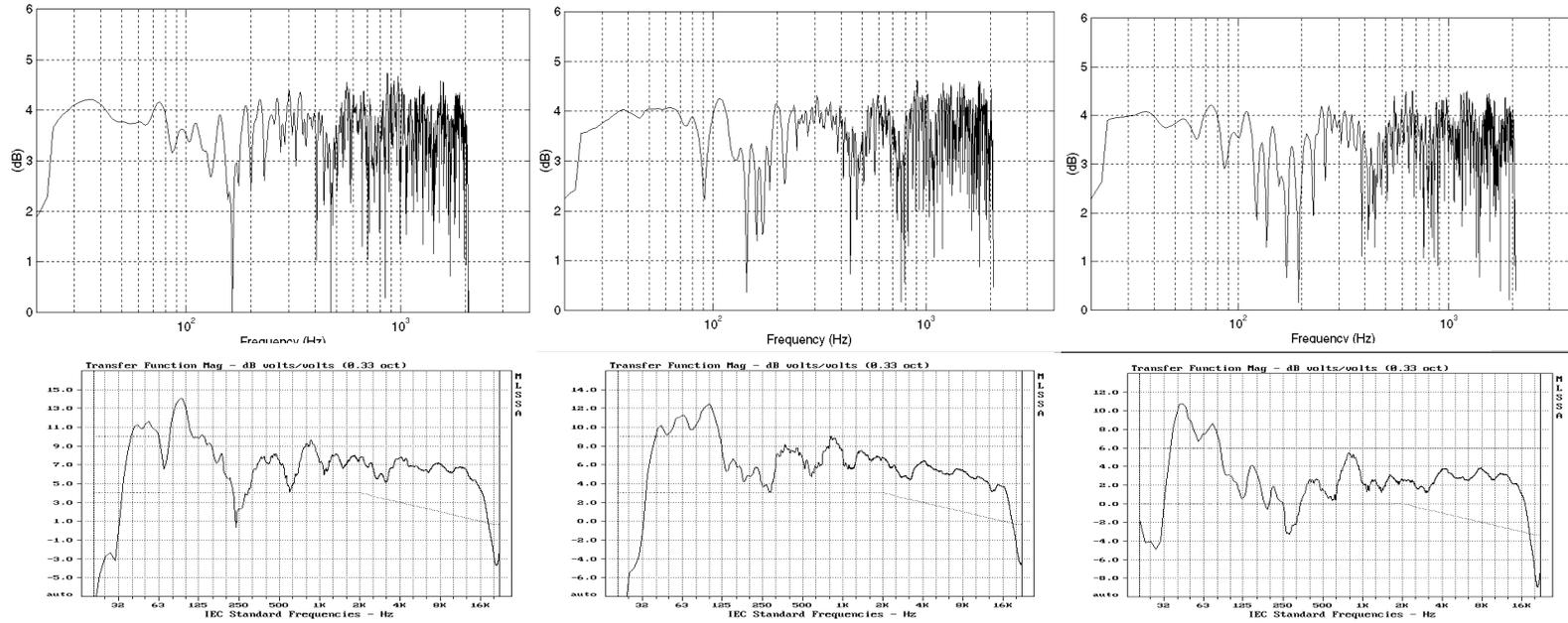
Fig.10. Measured and predicted transfer functions (FL, FC, FR)
