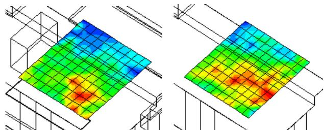
Figure 8. Central gravity time around the listening point, with and without furniture at 1000Hz
