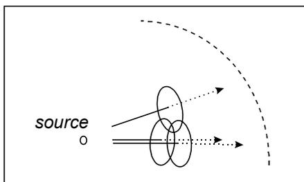
Figure 3. Cone-tracing method
