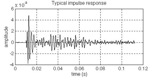
Figure 10. A typical room impulse response
