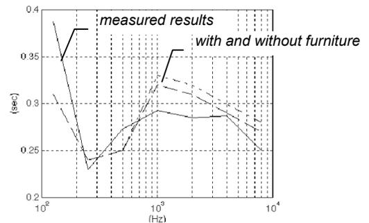
Figure 7. Statistical reverberation times ( $RT_{60}$ )
