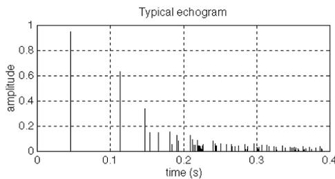
Figure 9. A typical echogram (e.g. at 1kHz)
