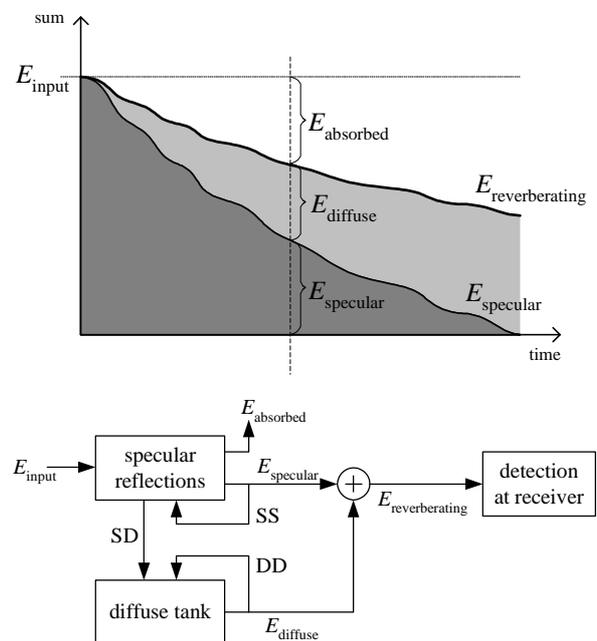
Figure 2: The ‘diffuse tank’ approach.
